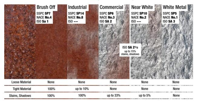
**NOTE:** Refer to Item 6 for larger samples of photos that can be used to match to the surface you are preparing.
