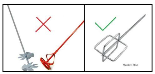
A drill-operated stirrer must not have sharp edges because these will scrape plastic shards off the bucket which will end up in the coating.
